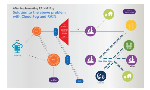
Here RAIN is behaving like an application, where a request is made and is fulfilled if it is available, if not it will approach the Fog center to fulfill the request. Fog acts as an intermediate layer between the Edge devices and the Cloud. Edge devices request storage and communication services from the Fog and persistent storage to the cloud that will be communicated consequently as per demand and failover.
